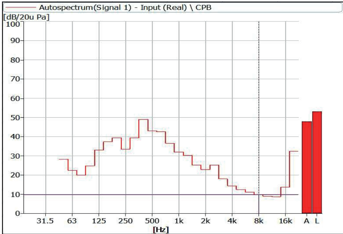
Figure 31 Noise Spectrum of Stage Luminaires (The Super Silence mode, Dynamic, No 1)
