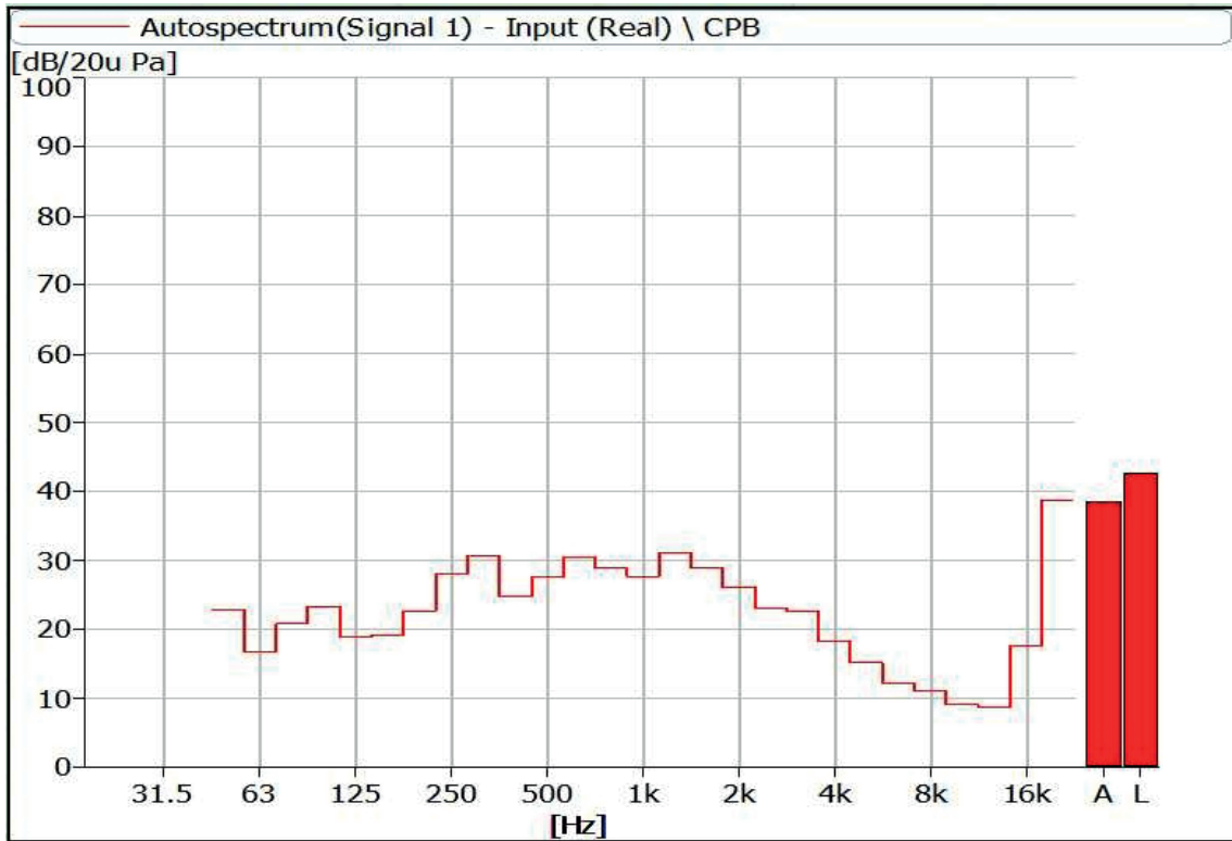
Figure 11 Noise Spectrum of Stage Luminaires (The Stage mode, Static, No 1)
