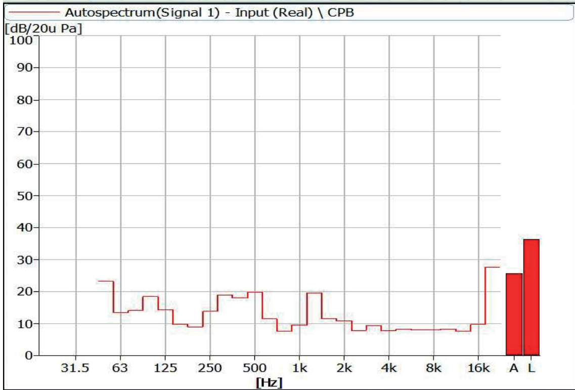
Figure 27 Noise Spectrum of Stage Luminaires (The Super Silence mode, Static, No 1)
