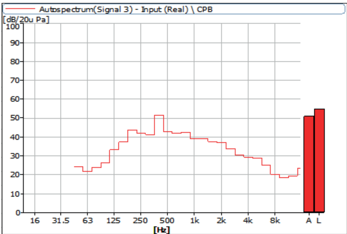
Figure 10 Noise Spectrum of Stage Luminaires (The Auto mode, Dynamic, No 4)
