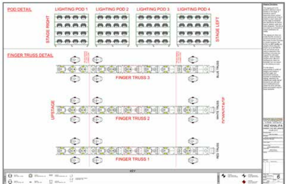
Plot details showing on the three finger trusses and the MagicPanel pods from the US tour.
