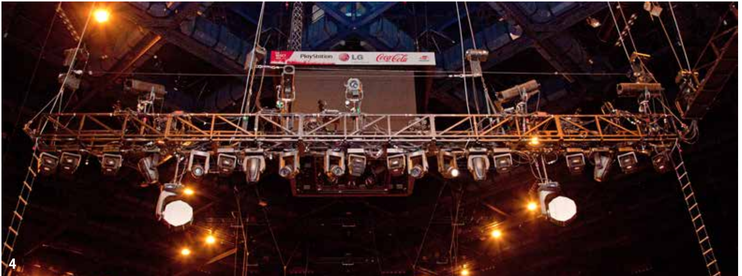
4. The downstage FlipBox™ truss, with Robert Juliat Topaze followspots on top, shown at Bruce Springsteen and the E-street Band's show in Paris - Ready to rock!
