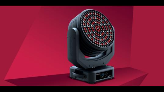
The proprietary, silicone-based, high-output 6:1 optical zoom ensures perfect colour stability over time, with a zoom range of 10° to 60°. The transmitting lens is equipped with an integrated honeycomb "egg crate" louver to prevent unwanted off-axis glare.
