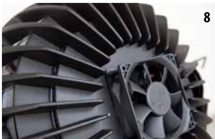
7. The Salad Bowl! The cast aluminium frame, which is the backbone of the head of the device: a very attractive piece!
